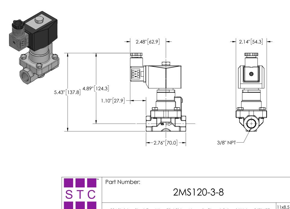
304 Stainless Steel, Two-Way, Pilot Piston, Normally Closed, Solenoid Valve, 3/8" NPT
