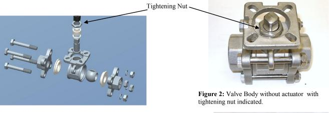
Figure 1: Exploded view of valve body with tightening nut indicated.
