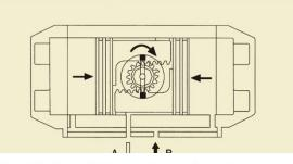
Air into Port B forces the pistons inwards, causing the pinion to turn clockwise while the air is being exhausted from Port A.
