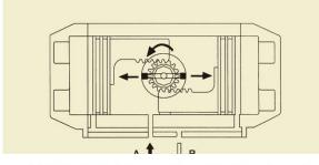
Air into Port A forces the pistons outwards, causing the pinion to turn counterclockwise while the air being exhausted from Port B.
