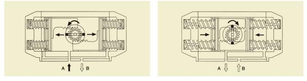
Air into Port A forces the pistons outwards, causing the springs to compress, the pinion turns counterclockwise while air is being exhausted from Port B. In the event of loss air pressure or power, the stored energy in the springs forces the pistons inwards, causing the pinion turns clockwise while air is being exhausted from Port A, and air to Port B can accelerate closing the valve.
